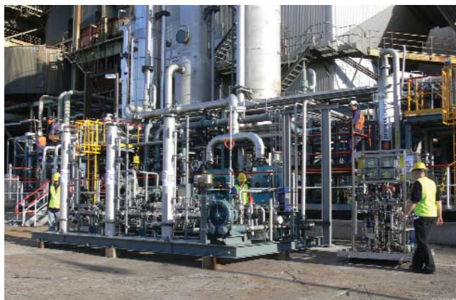
Vacuum swing adsorption is one of three carbon dioxide separation technologies being evaluated through the CO 2 CRC H3 Capture Project. (Image: CO 2 CRC)
