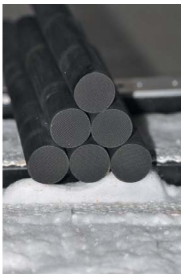
Figure 1: (LEFT) The VeloxoTherm™ structured adsorbents developed by Inventys; (RIGHT) conventional granular adsorbent.
