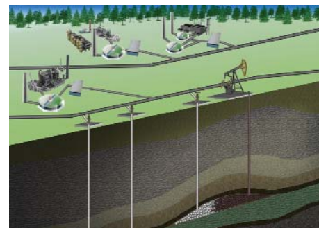
Figure 4: Enhanced oil recovery using the VeloxoTherm process. Carbon dioxide is captured from a flue gas generated from a variety of industrial sources is injected into oil reservoirs to facilitate tertiary extraction of oil
